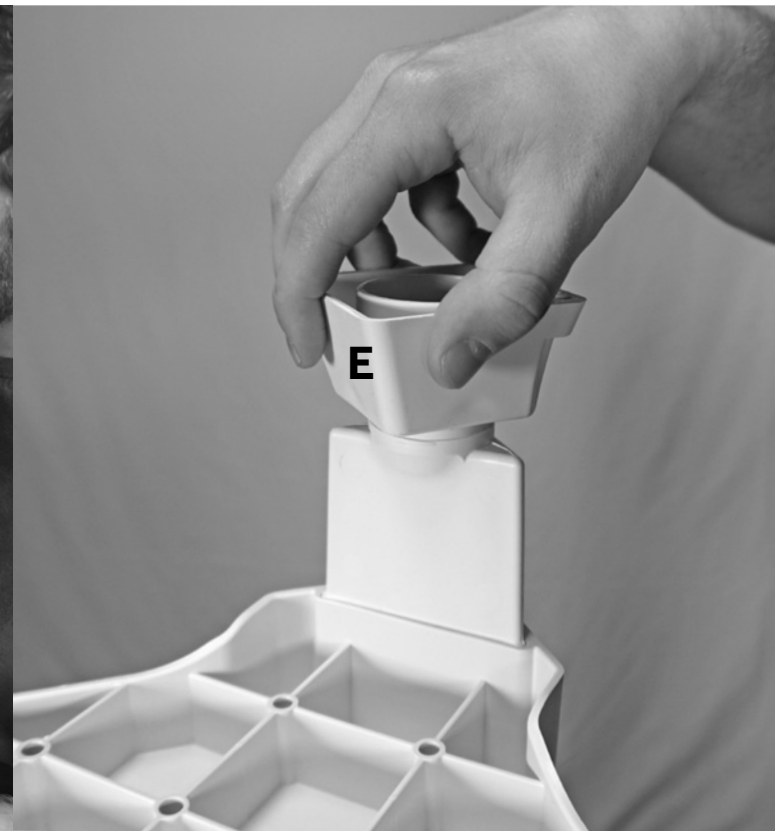
5 Screw the sink feet (E) onto the lower legs (D) by hand until tight. You will be able to unscrew each foot as needed to level the sink on an uneven floor once it is in its final position.
